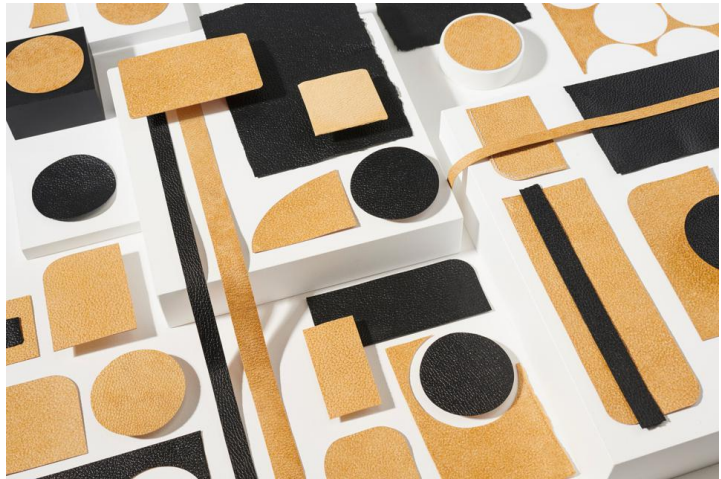
Compared to animal leathers that take at least a year to produce, mushroom-based Mylo is made in two weeks, with less petrochemicals than non-animal leathers. BOLT THREADS
